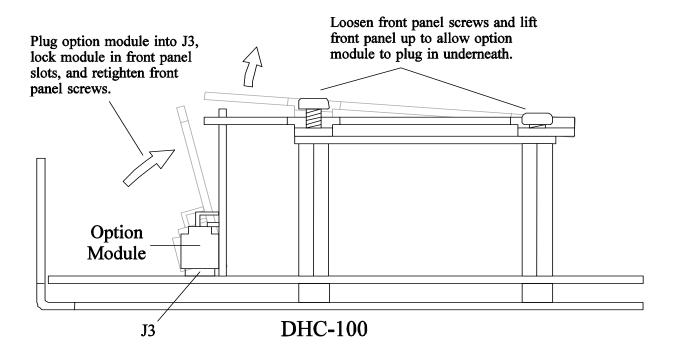
Installing an Option Module
