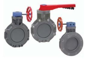
Spears<sup>®</sup> innovative design departs from traditional liner-seat type valves to eliminate seat creep, reduce operating torque and provide positive seal off. Ideally suited for flow control or throttling, this high performance valve is offered with a full variety of options for greater application versatility. Standard valves are produced from PVC or high temperature CPVC in IPS sizes 1-1/2" through 14". PVC and CPVC True Lug valves are produced in sizes 1-1/2" through 12".
