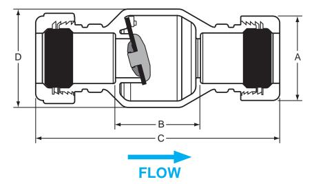
WARNING: The compression joints provide a positive seal but do not restrain pipe from thrust and movement under pressure. Use of compression joint requires blocking of connecting pipe to prevent any movement. Failure to do so can result in system failure or severe personal injury. Use in cold water/fluid applications only.
