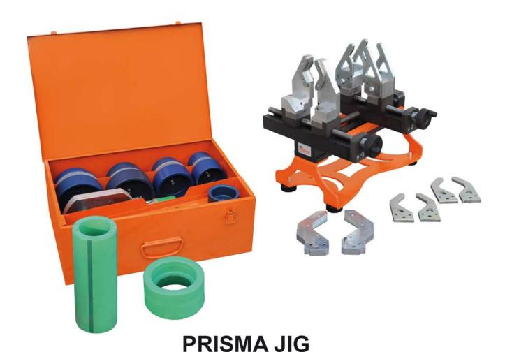
The PRISMA JIG is a compact socket welding machine for HDPE, PP and PP-R, PVDF, PB OD  $20^* \div 125$  mm (standard composition steel clamps from Ø 63 to 125 mm; on request from Ø 20 to 63 mm). The machine displays a steel frame that can be used as a support to the aligning body; the unit distinguishes itself by being able to work in tight spaces, after a swift releasing manoeuvre of the frame.
